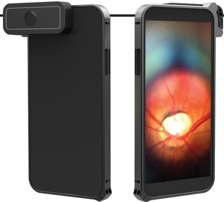
The D-EYE imager attaches to a smartphone with a sleek bumper that positions the lens over the phone's existing camera and light source.
